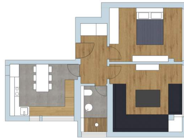
LAYOUT 1 - simplest option as the layout remains almost unchanged apart from the kitchen/dining becoming open plan
